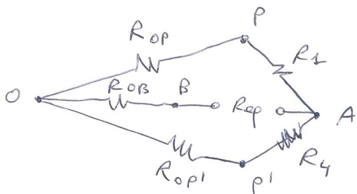
$$R' = (R_{op} + R_1) // (R_{op1} + R_4)$$
