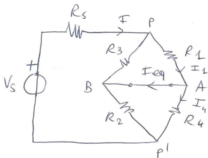
$$I = \frac{V_s}{R_s + \frac{R_1 R_3}{R_1 + R_3} + \frac{R_2 R_4}{R_2 + R_4}}$$
