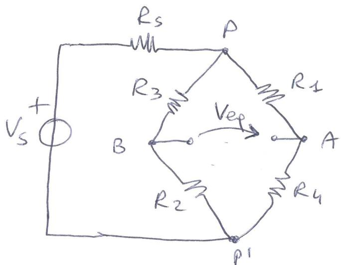
$$V_{PP'} = \frac{(R_1 + R_n) \parallel (R_2 + R_3)}{R_s + (R_1 + R_n) \parallel (R_2 + R_3)} V_s$$
