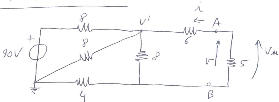
$$R_{eq} \Rightarrow \left\{ \left[ \frac{8}{18+4} \right] \parallel 8 \right\} + 6 = \\ \left\{ \frac{8}{18} \right\} + 6 = 10 \Omega$$
