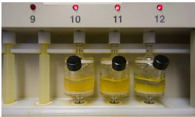
Fig. 2a. Fully auto- mated reactor for parallel small-scale SPPS, reaction vessels.
