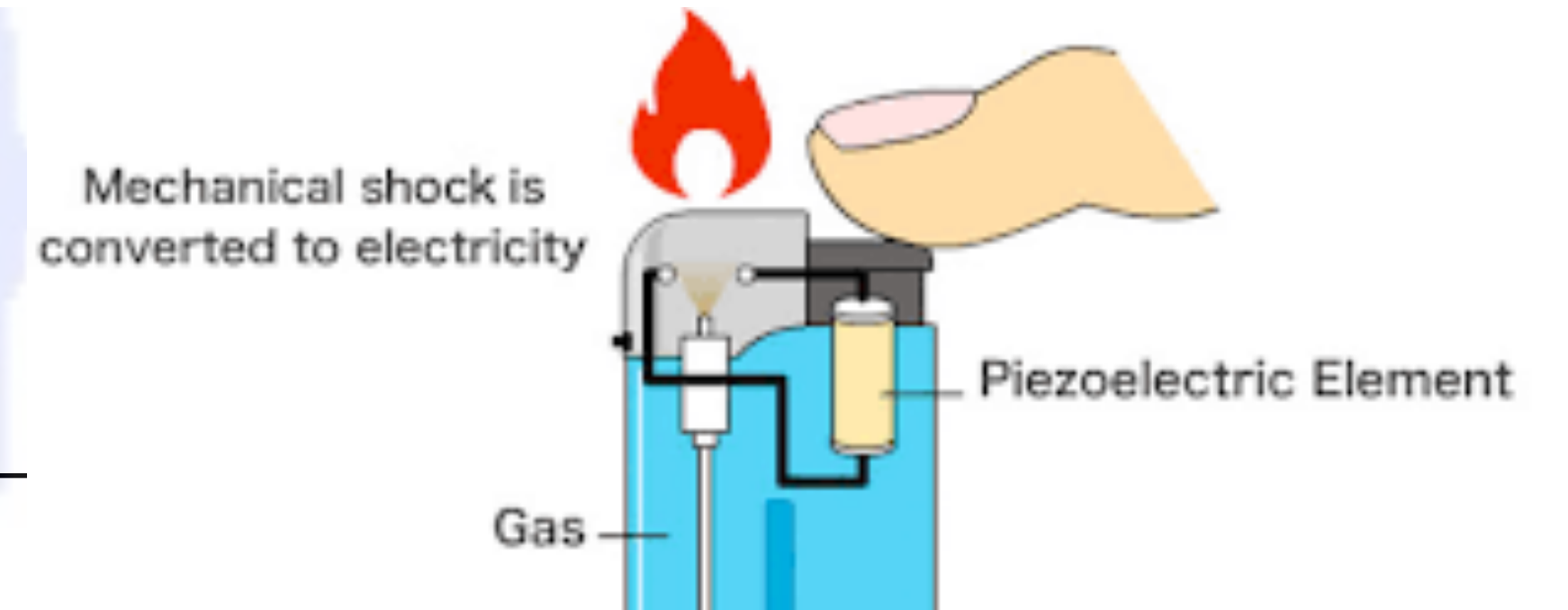
a) Direct Piezoelectric Effect
