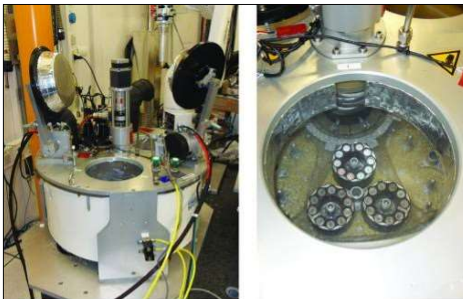
Figure 1: Automatic mounting system of the beamline MASSIF-1 of the ESRF (European Synchrotron Radiation Facility) synchrotron in Grenoble.
