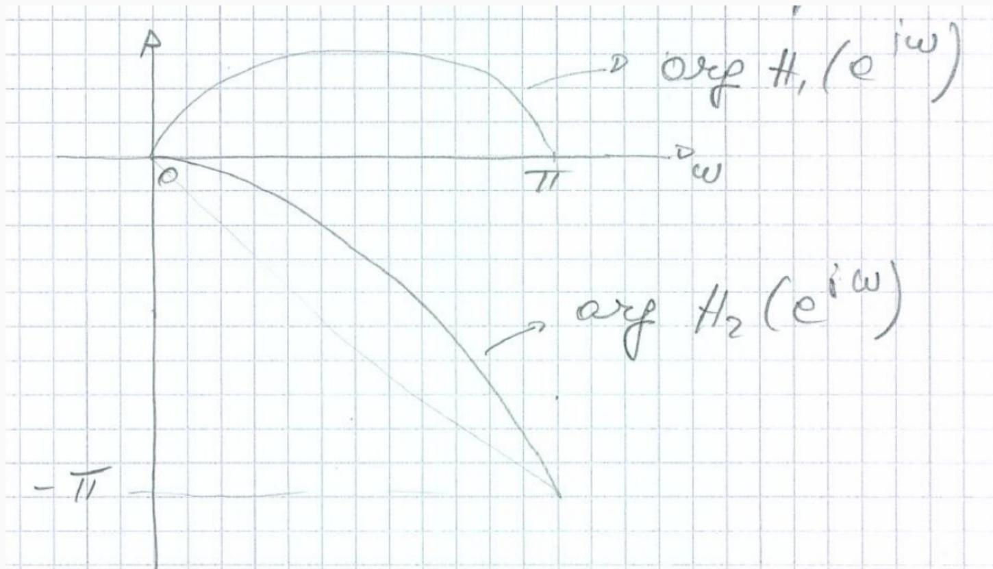
$$\arg [H_1(e^{j\omega})] = \theta_1(\omega) = \arctan \frac{\sin(\omega)}{b + \cos(\omega)} - \arctan \frac{\sin(\omega)}{a + \cos(\omega)}$$
