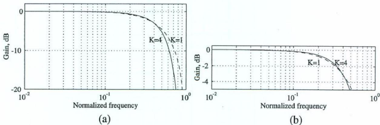
**Figure 4.23:** (a) Gain responses of a single first-order lowpass filter ( $K = 1$ ) and a cascade of four identical first-order lowpass filters ( $K = 4$ ) with a 3-dB cutoff frequency of  $\omega_c = 0.4\pi$ . (b) Passband details.
