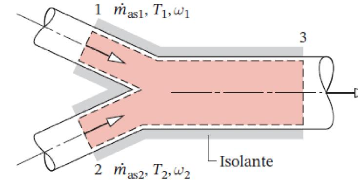
$\dot{m}_{da1} \cdot (h_{da1} + w_1 h_{vap,1}) + \dot{m}_{da2} \cdot (h_{da2} + w_2 h_{vap,2}) = \dot{m}_{da3} \cdot (h_{da3} + w_3 \cdot h_{v3})$  $w_1 \dot{m}_{da1} + w_2 \dot{m}_{da2} = w_3 \dot{m}_{da3}$  $\dot{m}_{da1} + \dot{m}_{da2} = \dot{m}_{da3}$
