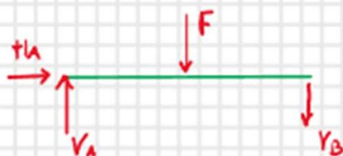
$$\begin{aligned} H_A &= 0 \\ V_A &= F/2 \\ V_B &= -F/2 \end{aligned}$$
