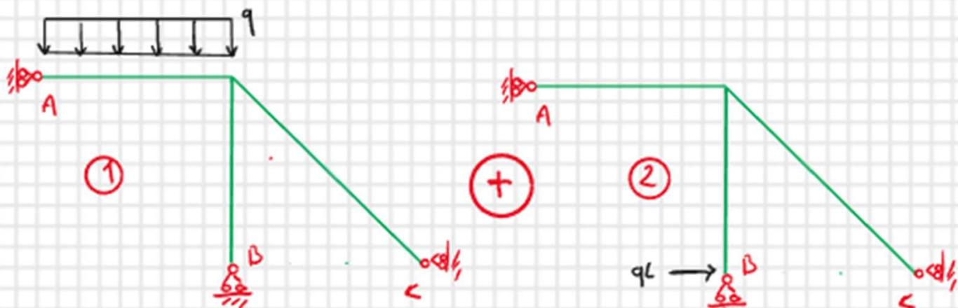
$$\left\{ H_A^1 = q\frac{L}{2} \quad V_B^1 = qL \quad H_C^1 = -\frac{qL}{2} \right\} + \left\{ H_A^2 = 0 \quad V_B^2 = 0 \quad H_C^2 = -qL \right\}$$
