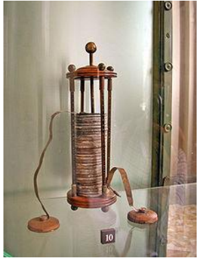
First prototype of battery in history (Cu/Zn, 1800)
