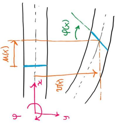
$u_x(x, y)$  DISPLACEMENTS OF THE GENERIC POINT  $(x, y)$  OF THE BEAM
