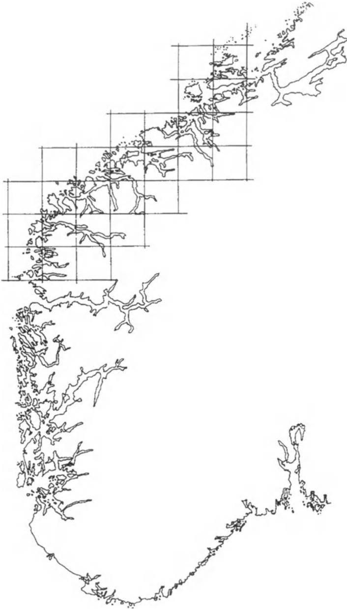
**FIGURE 5.11** The coast of the southern part of Norway. The outline was traced from an atlas and digitized at about  $1800 \times 1200$  pixels. The square grid indicated has a spacing of  $\delta \sim 50$  km. [Reprinted from Feder, *Fractals*, Plenum Press, p. 7.]
