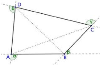
$$\begin{aligned} \alpha &= \widehat{ABD} + \widehat{ADB} \text{ guardando } ABD^\Delta \\ \beta &= \widehat{BAC} + \widehat{ACB} \text{ guardando } ABC^\Delta \\ \gamma &= \widehat{BDC} + \widehat{DBC} \text{ guardando } CBD^\Delta \\ \delta &= \widehat{DAC} + \widehat{ACD} \text{ guardando } ACD^\Delta \\ \alpha + \beta + \gamma + \delta &= (\hat{A} + \hat{B} + \hat{C} + \hat{D}) = \text{angolo piatto} \end{aligned}$$
