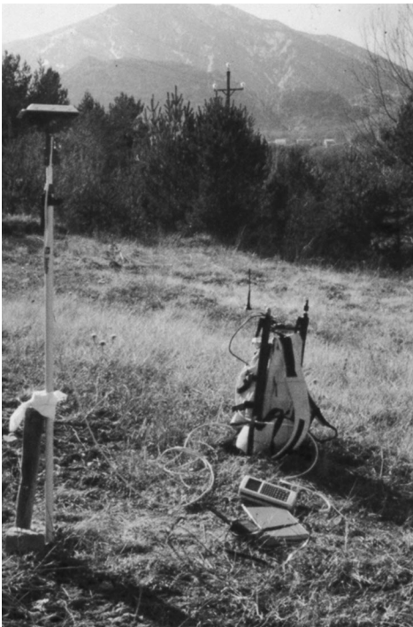
Fig. 13. Different set-up methods in Vallcebre monitoring points. (a) Telescopic pole with auxiliary tripod at point G1, an iron pin in a rock block. (b) At point G15, a wood stake in soil, the telescopic pole could be maintained vertical by hand for RTK positioning. The GPS receiver is in the yellow backpack and is controlled by means of the data collector TDC1 beside the notebook and the walkie-talkie. At the backpack top, the small black antenna of the UHF data link receiver can be identified. (c) Set-up with tripod having optical plummet over an inclinometer borehole, B1.
