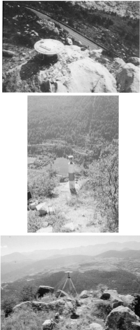
Fig. 5. Different antenna set-up in Vallcebre and Pont de Bar (Spain) base points: (a) antenna directly over a rock outcrop; (b) station over a concrete cylinder; (c) set-up with tripod having optical plummet. The GPS receiver, in the yellow case on the ground at the left in (b) and (c), is connected to the antenna through a signal cable. The plane dish around the antenna that can be seen in (a) and (c) is the ground plane that reduces the multipath error.
