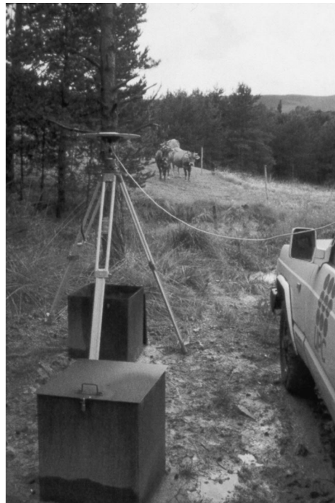
Fig. 13. Different set-up methods in Vallcebre monitoring points. (a) Telescopic pole with auxiliary tripod at point G1, an iron pin in a rock block. (b) At point G15, a wood stake in soil, the telescopic pole could be maintained vertical by hand for RTK positioning. The GPS receiver is in the yellow backpack and is controlled by means of the data collector TDC1 beside the notebook and the walkie-talkie. At the backpack top, the small black antenna of the UHF data link receiver can be identified. (c) Set-up with tripod having optical plummet over an inclinometer borehole, B1.
