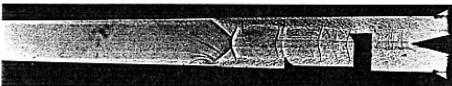
Multiple bifurcated shocks in the duct of Plate B,5b at still higher Mach number. M = 1.70 .
