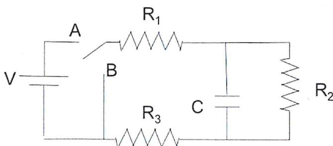
2. Consideriamo il circuito in figura, con  $C=1.90$  nF,  $V=12.0$  V,  $R_1=10.0$  k $\Omega$ ,  $R_2=15.0$  k $\Omega$ ,  $R_3=20.0$  k $\Omega$ . Calcolate:
