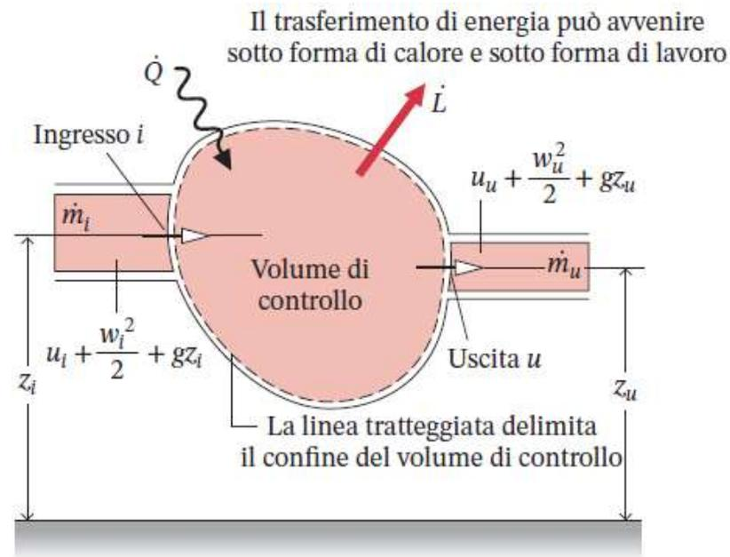
$$\frac{dE_{vc}}{dt} = \dot{Q} - \dot{L} + \dot{m}_i \left( u_i + \frac{w_i^2}{2} + gz_i \right) - \dot{m}_u \left( u_u + \frac{w_u^2}{2} + gz_u \right)$$
