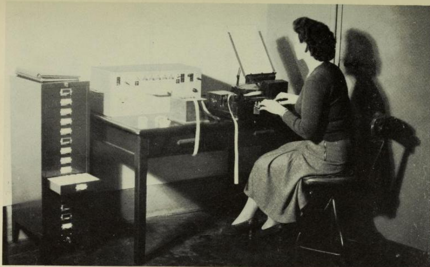
The library of tapes on which subroutines are punched is contained in the steel cabinet shown on the left. The operator is punching a program tape on keyboard perforator. By placing library tapes on the tapereader shown in the center of the photograph, the operator can copy them mechanically onto the tape she is preparing.
