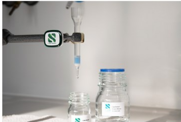
Fig. 8: A drip column filled with our INDIGO agarose. The agarose filled in this columns have big diameters to prevent the column from clogging.
