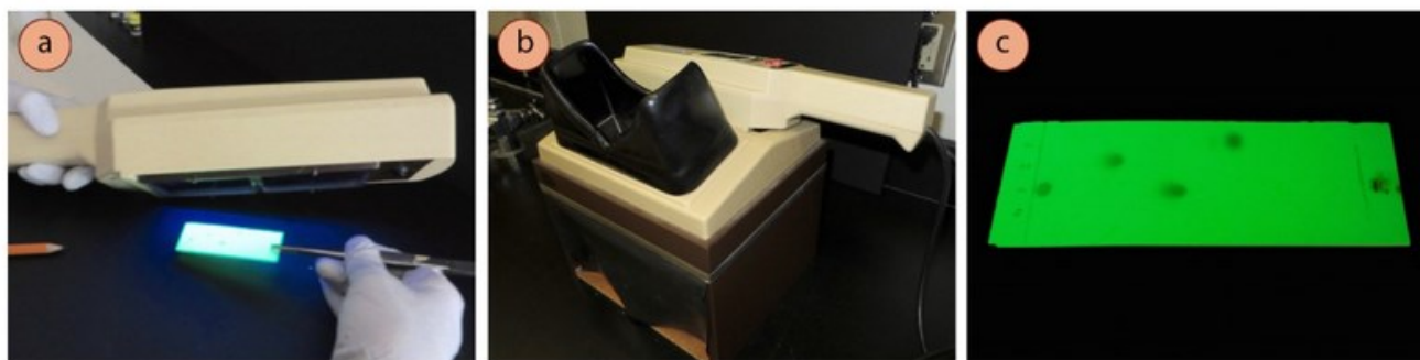
Figure 2.31: a) Tilting a UV lamp to visualize a TLC plate, b) Box to protect eyes from UV damage, c) Appearance under UV.
