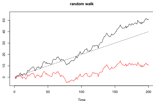
Figure 16: Normal Random Walk with p_0 = 0 , \sigma_w = 1 , with drift \delta = 0.2 (upper jagged line); without drift, \delta = 0 (red line). The dashed line is the straight line 0.2t .
