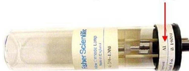
A hollow cathode lamp for Aluminum (Al)
