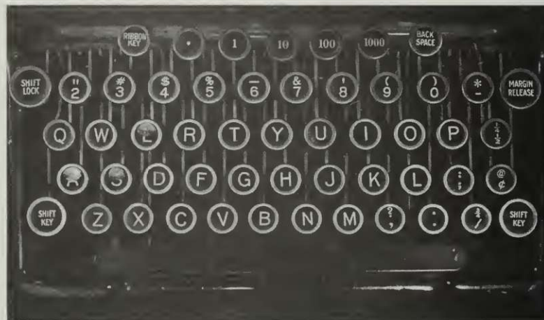
Notice the patterns of wear for most frequently used keys, as illustrated by breakage through the surface after so many years of striking. In QWERTY, all the most common keys are either not in the home row, or are hit by weak fingers in the home row—thus illustrating the suboptimality of this standard arrangement.
