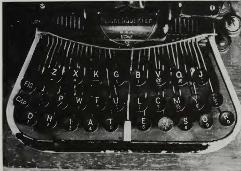
A keyboard for a typewriter made in the 1880's, illustrating one of the many competing non-QWERTY arrangements so common at the time.
