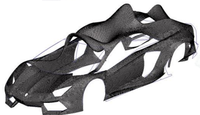
Modal analysis of the body of a Lamborghini Aventador
