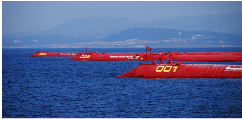
Fig. 15. The three-unit 3 \times 750 kW Pelamis wave farm in calm sea off northern Portugal, in 2008 (courtesy of R. Barros).
