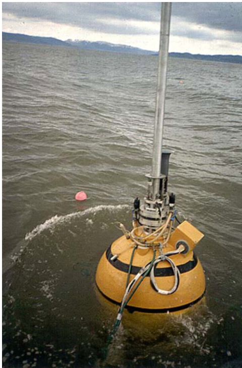
Fig. 7. Norwegian heaving buoy in Trondheim Fjord, 1983 (courtesy of J. Falnes).
