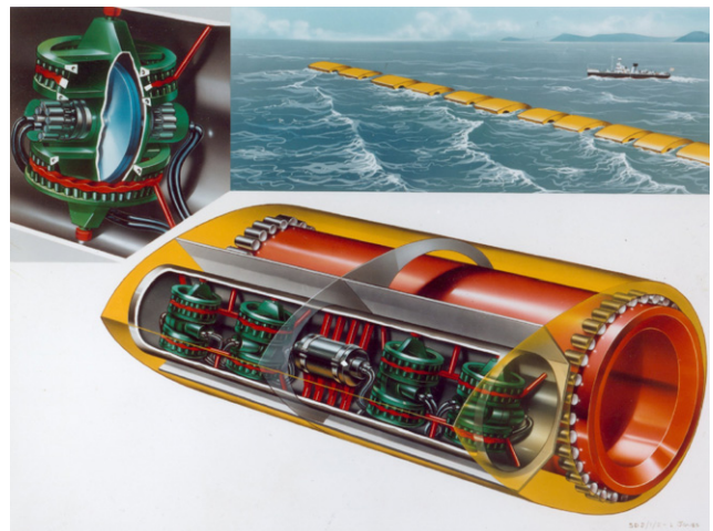
Fig. 14. The Duck version of 1979 equipped with gyroscopes (courtesy of University of Edinburgh).
