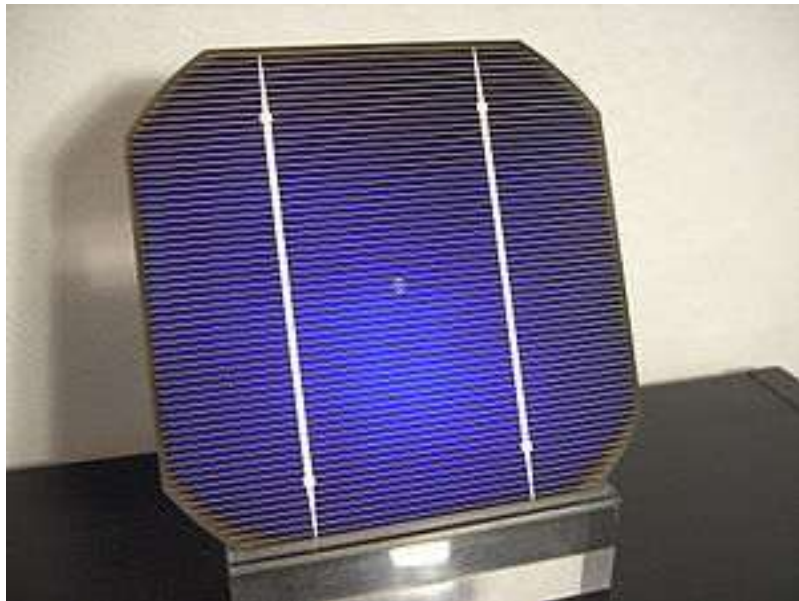
Cella in silicio monocristallino
