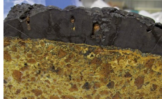
Cross-section of cobalt crust (SW Pacific)
