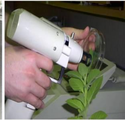
Gene gun Helios™ by BioRad is used to transfect cells in cultures and plant leaves
