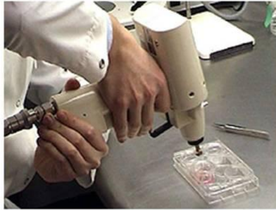
Gene gun Helios™ by BioRad is used to transfect cells in cultures and plant leaves
