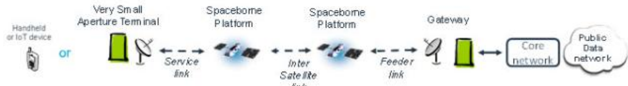
Figure 5: Satellite access network (with ISL) with a service link operating in frequency bands above 6 GHz [source: TR 38.811]
