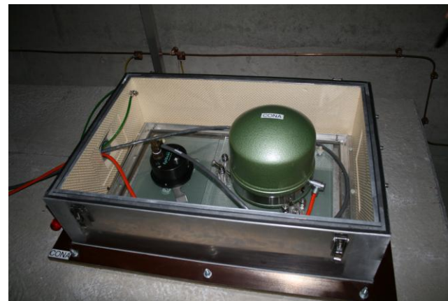
broad band seismometer
