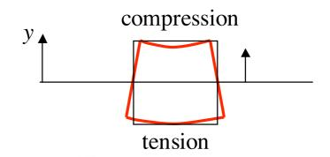
$$\left(\frac{\partial^4}{\partial x^4} - \frac{\rho A}{EI} \frac{\partial^2}{\partial t^2}\right) w = 0 \Rightarrow \omega = \pm k^2 \sqrt{\frac{EI}{\rho A}}$$
