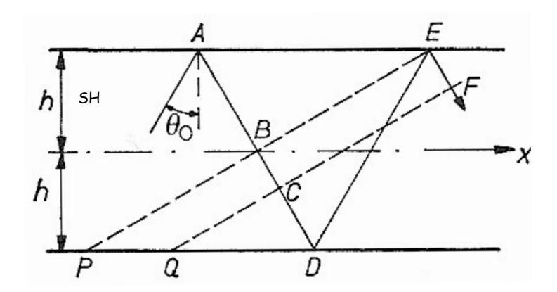
Repeated reflection in the layer allow interference between incident and reflected SH waves: SH reverberations can be totally trapped.
