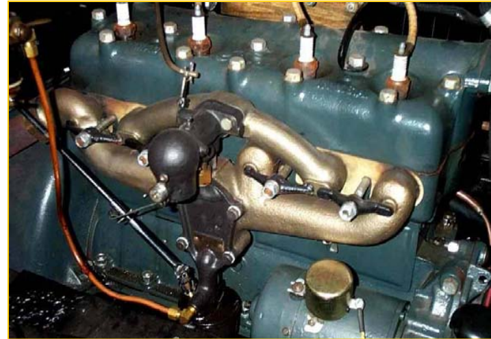
Engine Manifold coated with Pigmented Ceraset HTT
