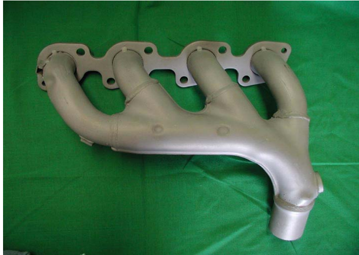
Heat exchanger coated with Ceraset HTT
