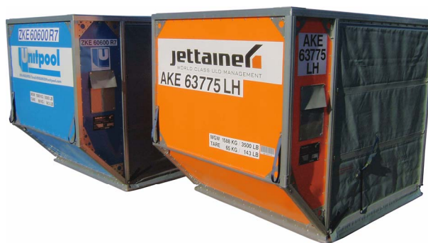
Figure 2. Two air cargo containers with panels made from gel-spun UHMWPE fibers and a Turane resin (Courtesy DoKaSch Aircargo equipment GmbH Staudt, Germany).
