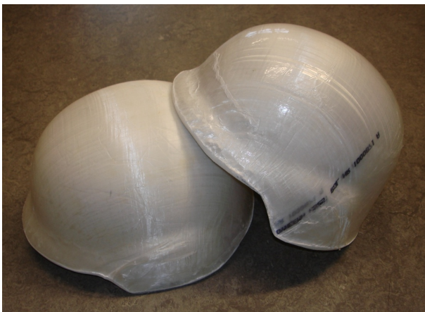
Figure 7. Two helmet shells made by creep-forming of gel-spun UHMWPE fibers [14].
