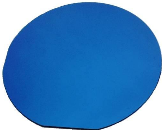
100 nm \text{Al}_2\text{O}_3 coating on Si wafer
