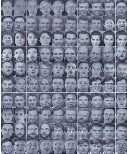
Figure 15.5: 100 training images. Each image consists of 92 \times 112 = 10304 greyscale pixels. The train data is scaled so that, represented as an image, the components of each image sum to 1. The average value of each pixel across all images is 9.70 \times 10^{-5} . This is a subset of the 400 images in the full Olivetti Research Face Database.
