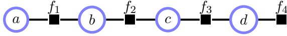
Figure 5.2: For singly connected structures without branches, simple messages from one variable to its neighbour may be defined to form an efficient marginal inference scheme.
